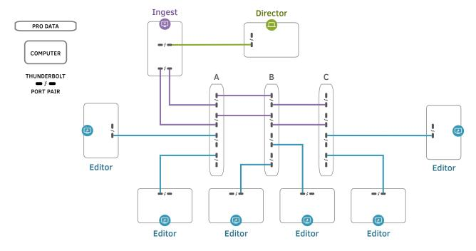
Ingest is dual-pathed for ultimate performance to all three Pro Data devices via daisy-chain, handing off containers to six Editors in teams of two per device. Director laptop is connected to the Ingest station via Thunderbolt-over-IP.
