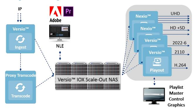
Adobe Premiere Pro CC editing coupled with Versio IOX Scale-Out NAS provides an affordable, industry-standard editing and storage system. This system leverages Versio IOX Scale-Out NAS with no additional hardware required for high-resolution editing. This type of solution is ideal for systems requiring a smaller number of editing systems and is readily available for freelance editors.
