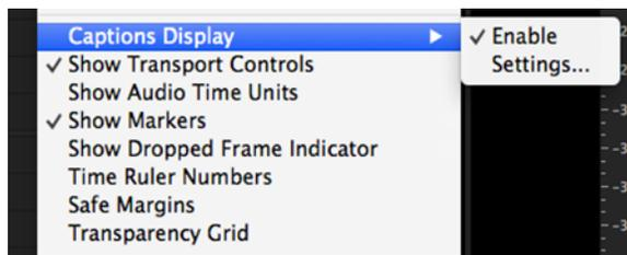
**NOTE:** Newer AJA hardware devices (for example, KONA 4 or Io 4K) Closed Captions will always be active for capture and playback. If, however, you are using earlier AJA hardware models, you must enable vertical ancillary data (VANC) using AJA Control Panel.
